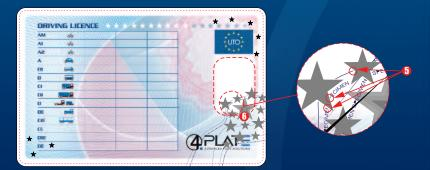
**5** Tight registration of **IDOPTIC**® with other features (Guilloche, microtext, CLI) forces counterfeiter to simulate several engraving methods and depths in register.
